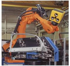
OptiCell - Precision non-contact robotic white light 3-D measurement
