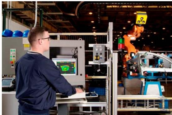
Ogihara installed its first OptiCell in mid 2007 and based on customers' requirements has over 50 different parts to measure as details and shipping units before delivery to the OEMs' assembly plants. Ogihara's unique process combines OptiCell's white light measurement technology with fast and agile laser welding systems installed at Ogihara's manufacturing facility. Ogihara complements detail part inspection with functional build applications to produce the best parts for its automotive
